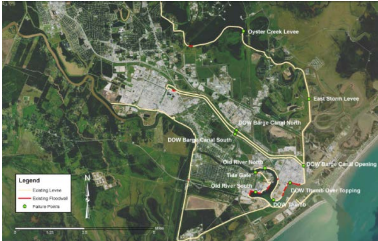
Figure 3-8: Freeport and Vicinity CSRM Failure Locations
