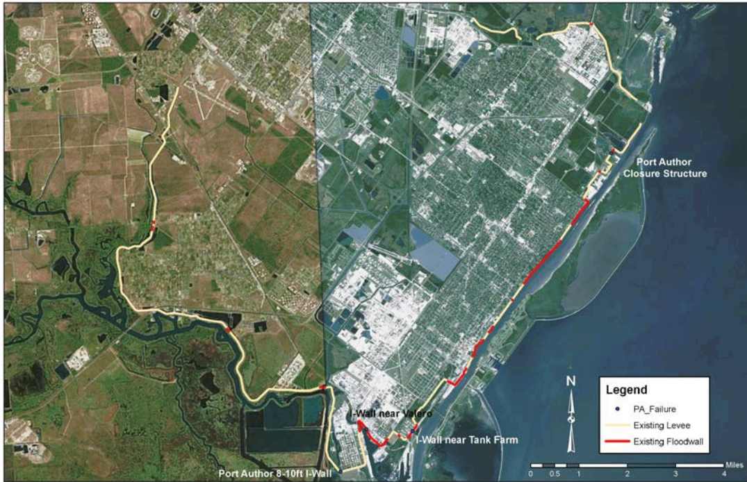
Figure 3-7: Port Arthur and Vicinity Failure Locations
