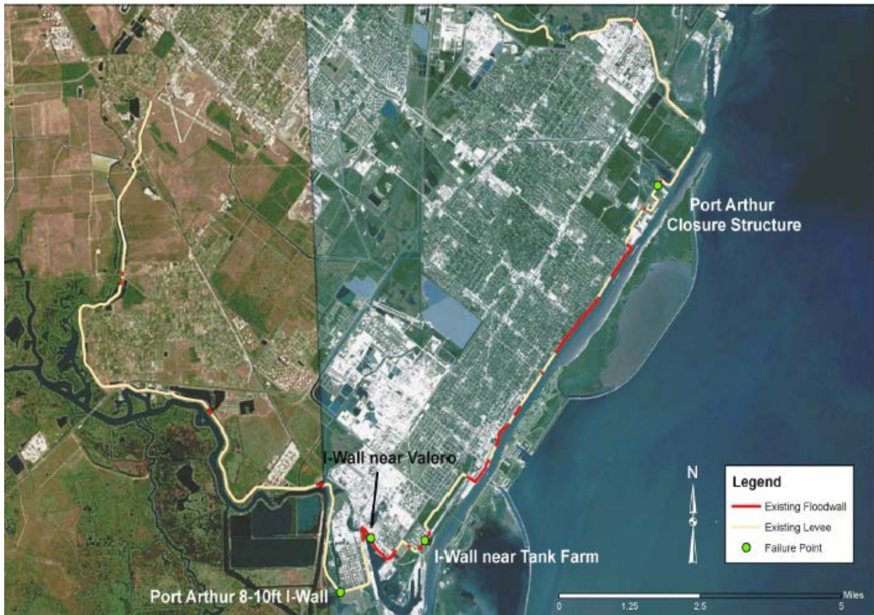
Figure 3-4: Port Arthur and Vicinity CSRM Failure Locations
