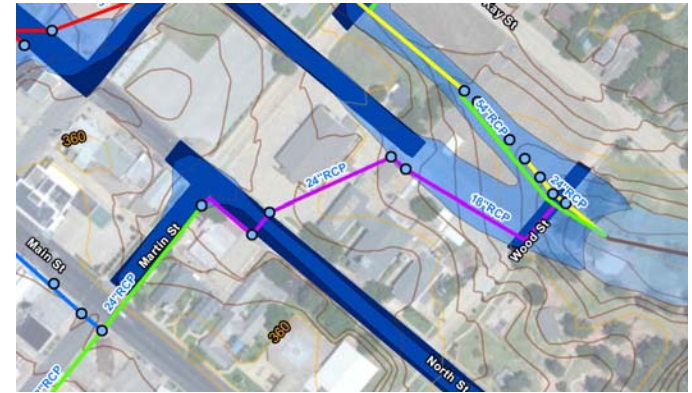
Existing bypass of the North Street system
