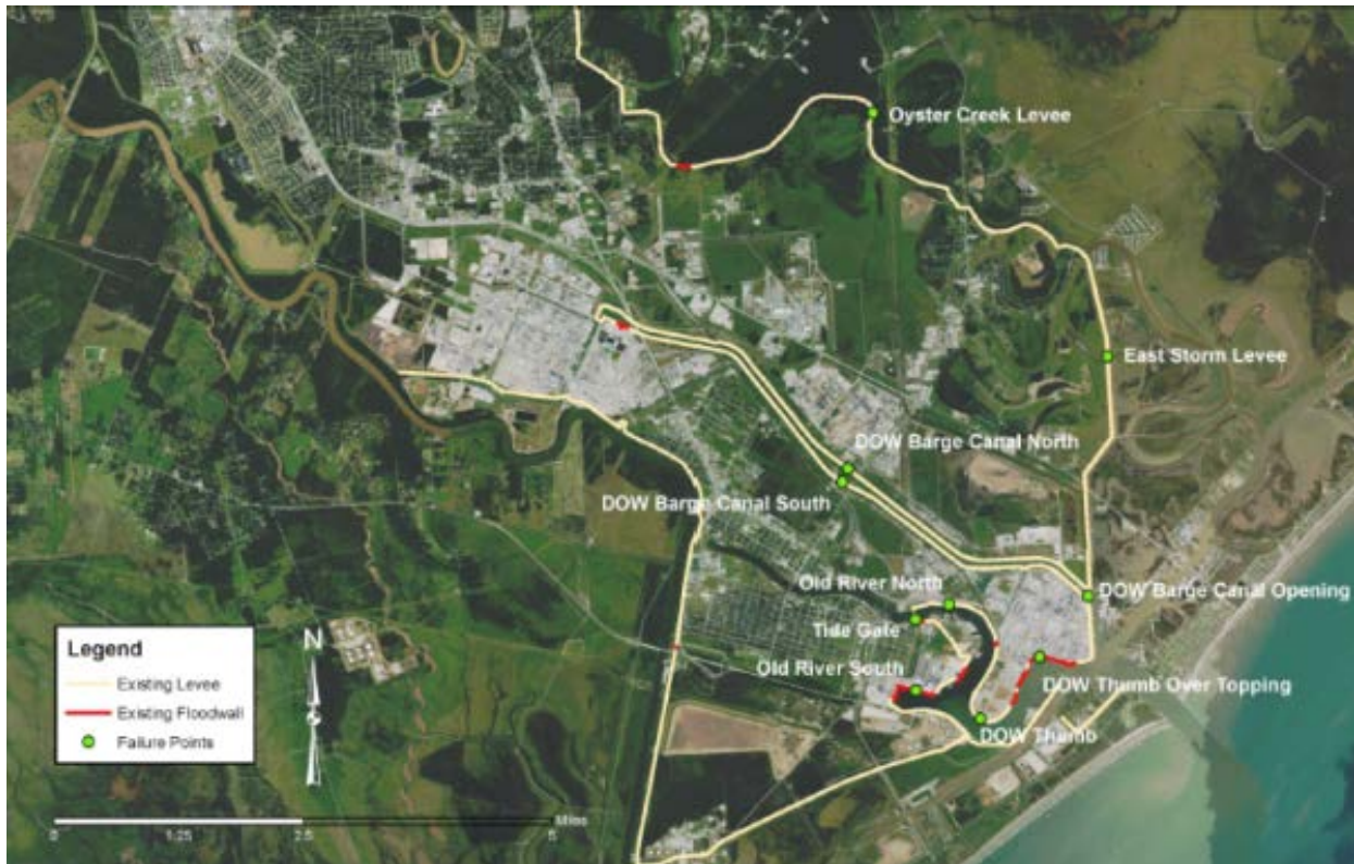
Figure 3-5: Existing HFPP in Freeport and Vicinity CSRM
